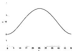
Fig. 13 Projections of the second mode shape on the x - z plane with crack depth of 30%
