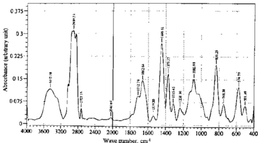
Figure 1. FTIR spectrum of HTLNR
