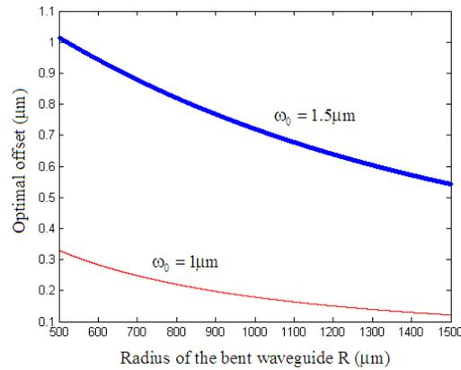
**Fig. 6** Optimal offset as a function of curved waveguide radii at different mode widths
