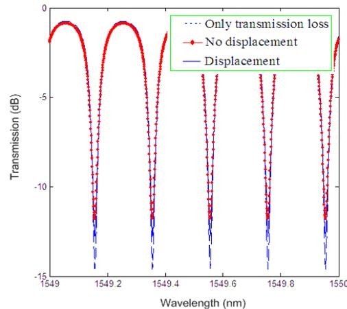
**Fig. 12** Transmission characteristics of the device for three cases (a) ideal case (only transmission loss) (b) no displacement of access waveguides and (c) with optimized displacement of access waveguides
