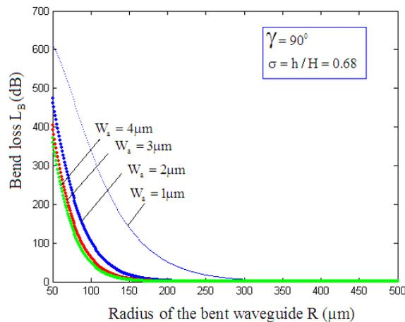
Fig. 4 Estimate of bend loss for a variety of waveguide widths
