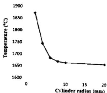
Figure 5 The relationship between temperature distribution and radius
