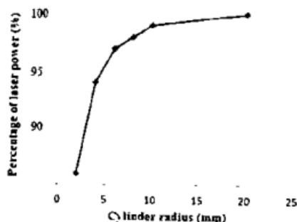
Figure 6 The trend of laser power changing with different radius
